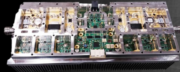
2.4GHz ISM, 2x250W Coherent, On-Board Exciter
